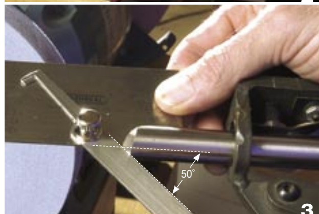
An inexpensive metal protractor will help you measure your tool bevels.
